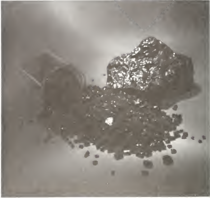
Solid solvent refined coal (SRC), a synthetic process which the Science Committee is funding, to remove sulfur and ash before the fuel is burned.
